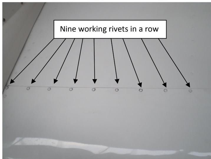
This was on the line where the front pre-formed leading edge of the stabilizer is riveted to the main skin and the front stabilizer spar. In addition *five* working rivets were found on the underside of the stabilizer on the same line. This in effect gives a total of fourteen working rivets in a line. There are also further random working rivets on the upper surface of the stabilizer.
