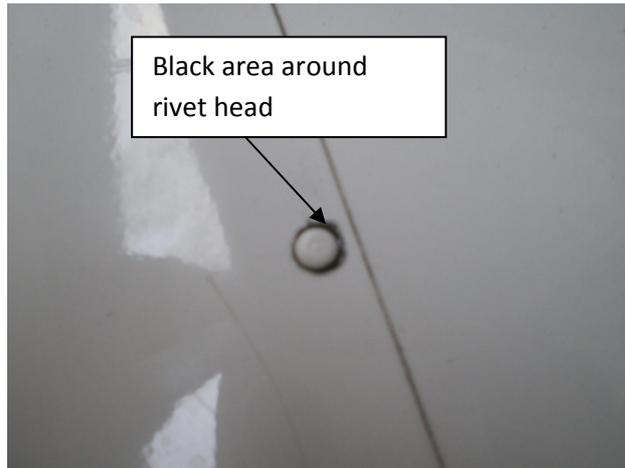
One or two working rivets are not considered cause for concern but several, especially in a row, are cause for concern. More than two adjacent working rivets in a row should immediately be investigated by a qualified aircraft sheet metal worker as this indicates a potential loss of structural integrity in that area. The following photograph shows nine working rivets in a row on the horizontal stabilizer of a C 152.
